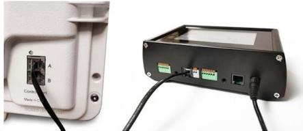
1). Connect one end of the RJ14 cord to the master controller A port, the other end to the A port of the light fixture.
