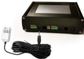
1). Connect the temperature sensor plug into the master controller temperature sensor port A. Hang the sensor at canopy height making sure the sensor and cord are hung and routed away from direct heat sources. Repeat install with port B, if necessary.
